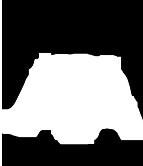
Figure 8.9: Mask after rounds of dilation to add back any of the main blocks that were eroded when removing noise
