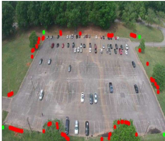
Figure 8.12: List of possible corners found shown in red with best corners highlighted in green
