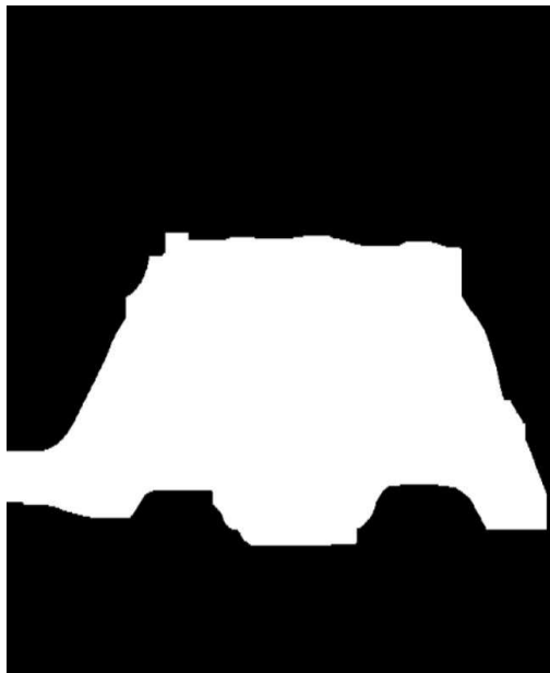
Figure 8.8: Mask after rounds of opening to further remove noise
